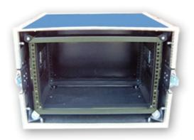
Flight Cases to house industry standard 19" rack mounted equipment made from Birch plywood faced with a high pressure laminate / phenolic finish available in many colours. Hardware includes steel ball corners, recessed catches and handles.
